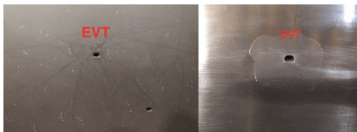
Picture 2. Far field mic hole on top cover.
